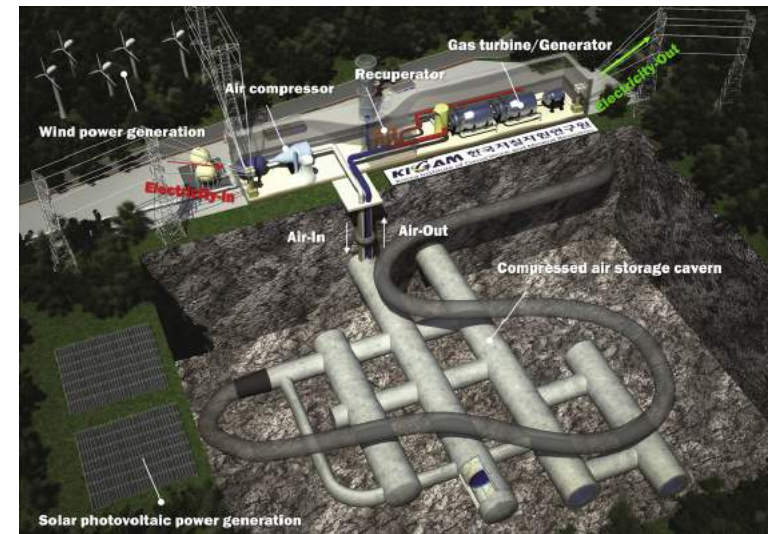
Components of an underground CAES system
